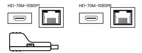
Connect a 5V power adapter via built-in micro-USB at HE1-70M-1080PT when the source doesn't provide enough power to the receiver.
